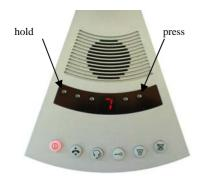
Hold down the "external volume" button. The display shows the current volume level for the extension (external loudspeaker).
