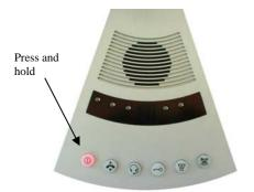
Press the on/off button for longer than 2 seconds.
