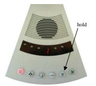
As long as the "Announcements/Paging" button is pressed, either the volume of the extension increased, or the announcement goes via a separate loudspeaker, which could e.g. be in a waiting room.
