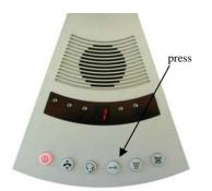
When the "door opener/switch contact" button is pressed, the connected function, e.g. a door opener, is controlled for about 3 seconds.
