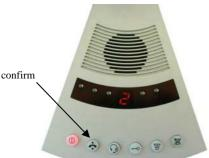
By pressing the "call receive" button, the existing connection is temporarily interrupted and you are connected to the selected extension.
