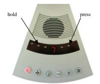
Hold down the "internal volume" button. The display shows the current volume level for the main control (internal loudspeaker).
