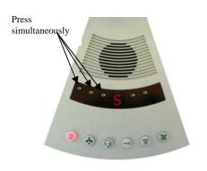
Press the external volume, internal volume and attenuation buttons simultaneously for about 3 seconds.
