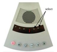
Use the + and – buttons to select the extension to which a connection is to be established. The number of the selected extension (e.g. no. "2") flashes faintly, alternating with the dark number of the current connection (e.g. no. "1").
