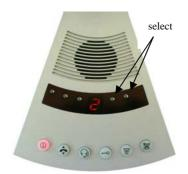
The value can now be modified using the + and buttons (in this case from "0" to "2").
