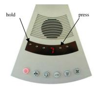
Hold down the "external volume" button. The display shows the current volume level for the extension (external loudspeaker).
