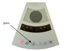
Press the "Headset On/Off" button to switch the intercom to headset operation.
