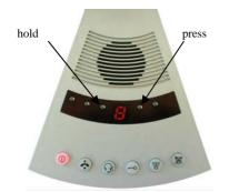
Hold down the "Attenuation" button. The display shows the current attenuation level (preset at "8").
