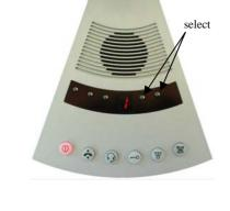
Use the + and – buttons to select the extension to which you wish to connect briefly. The number of the extension selected (2) flashes lightly, alternating with the dark number of the current connection (1).
